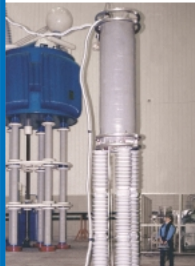
500kV REACTOR UNDER IMPULSE TEST
